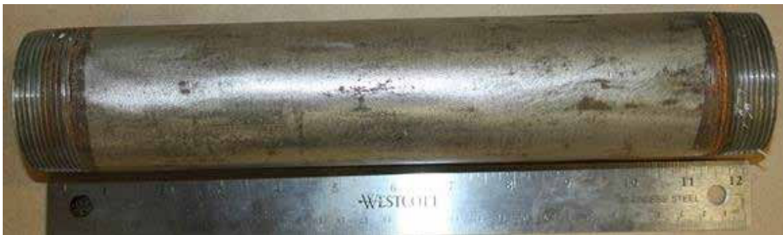
Fig.7.1: Pipe surface of continuous sweating test after the test with traces of corrosion (after cleaning).
