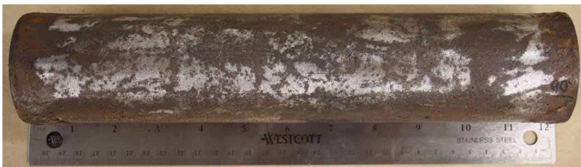
Fig.7.2: Pipe surface of high temperature cycle test after the test with traces of corrosion (after cleaning).
