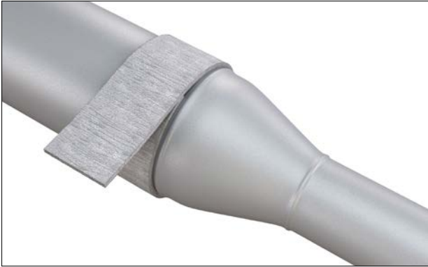
Figure 45: Measuring pipe circumference.
