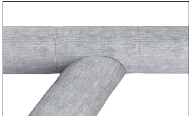
Figure 55: Completed tee cover.
