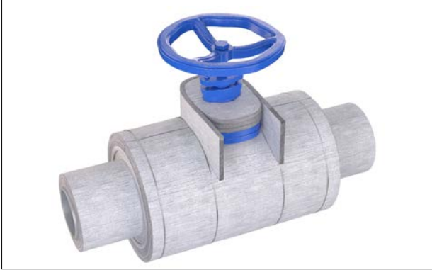
Figure 62: Fabricate spindle bonnet cap.
