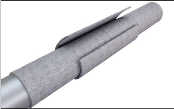
Figure 13: Staggering of next layer of ArmaGel.
