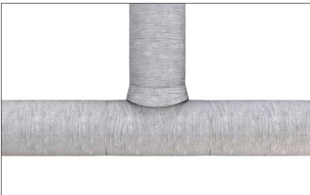
Figure 51: Installation of tee cover.
