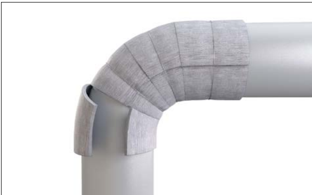
Figure 36: Securement of segments using insulation wire.
