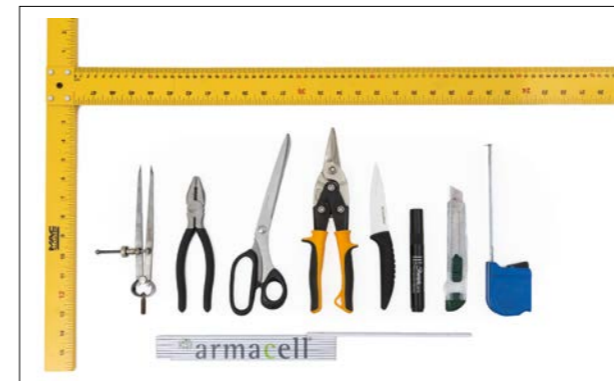
Figure 4: Recommended tools for application of ArmaGel DT
