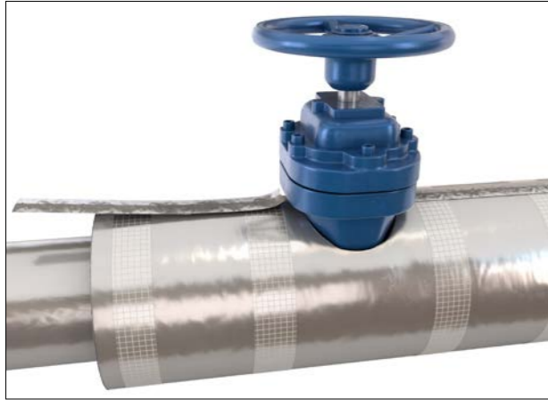
Figure 42: Application of vapour barrier tape
