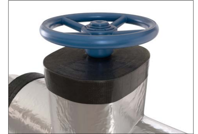
Figure 57: Application of vapour stop at spindle insulation termination
