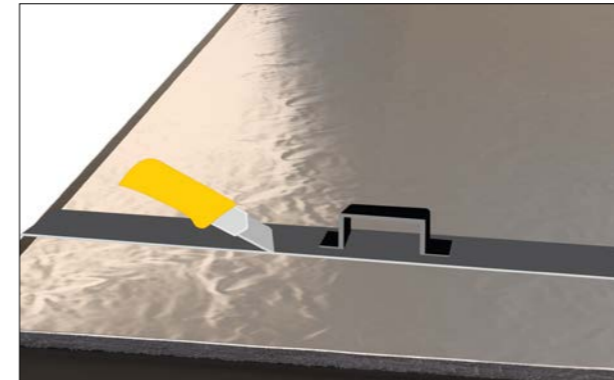
Figure 3: Prefabrication cutting in the workshop
