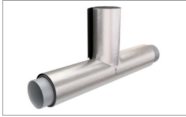
Figure 75: Application of primary vapour barrier on tee
