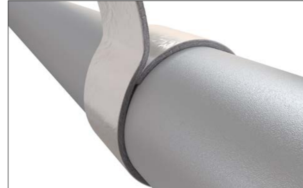
Figure 7: Determining the circumference of the pipe
