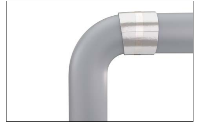
Figure 17: Application of starter segment
