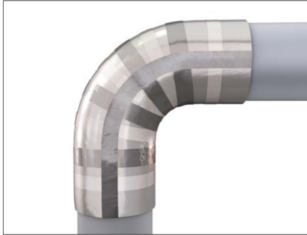
Figure 20: Fully secured vapour barrier tape
