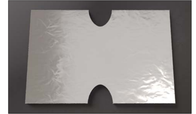
Figure 22: Equal tee fabrication
